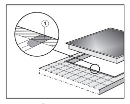
Grout lines ① and the hatched area underneath the hob frame must be smooth and even. If they are not the hob will not sit flush with the worktop and the sealing strip underneath the hob will not provide a good seal between the hob and the worktop.
